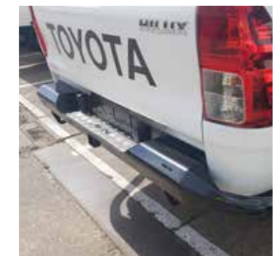
Pare-choc arrière en acier Replacement rear bumper bar HILUX D/C, S/C Ref. 20TF0081
