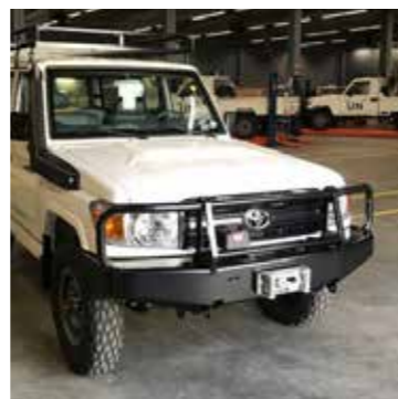
Pare-buffle renforcé, prise treuil
